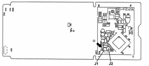
NOTE : For remodelling, take out the batteries and press the OPERATE/STOP(ON/OFF) button twice or 3 times at first. After finish remodelling, put back the batteries then press the RESET button.
